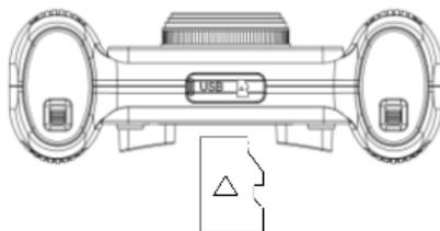
**Note: The camera is not equipped with built-in memory. Please insert a memory card before using. Before using the memory card for the first time it is necessary to format the card in the camera.**
