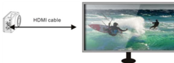
**Note: Before connecting or removing the HDMI cable, please stop video recording, playback and disconnect Wi-Fi first.**
