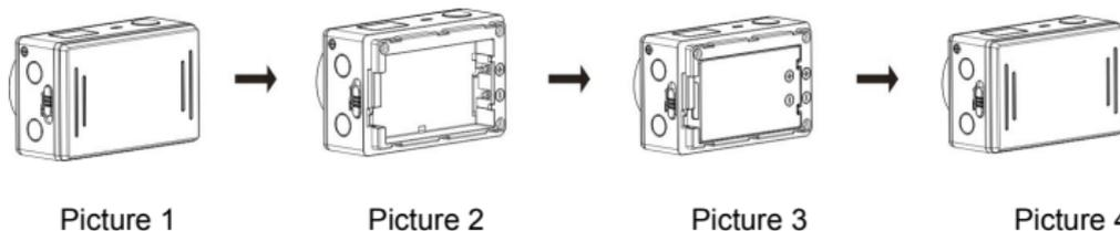
Step 1. Push the battery cover switch to the lock position(
