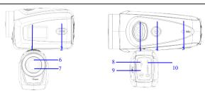
Black and white digital screen(2)MODE key(3)Shutter (4)Power(5) Microphone(6)Lens(7)Reset(8)USB port(9)TV port(0)TF card slot
