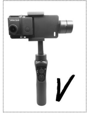
**Step 3:** Before turning on the gimbal, try to adjust the total weight as centred as possible so that the action cam adapter is slightly horizontal. You can adjust the weight distribution with the adjustable arm (12).
