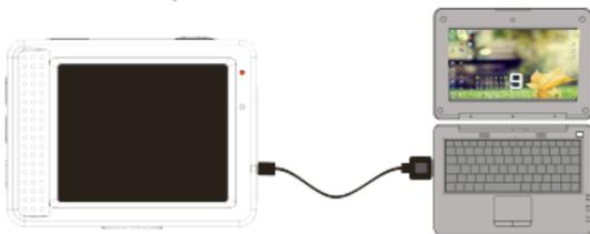
Connect the camera to computer for charging under shutdown status. The charging indicator will be on when charging, and will be off when the battery is fully charged. Generally, the battery can be fully charged after 2-4 hours.
