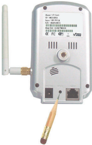
Figure 3-25: Stick on the reset button to set to the factory default
