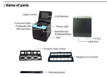
Ve strongly suggest using a clean, dry, non-alcohol cotton swab to insert into the film scanner slc nd clean the glass surface periodically to produce a clear image.
